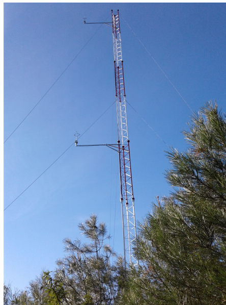
Figure 2.2 – Meteorological mast with two sonic anemometers deployed during the Perdigão 2017 experiment.
