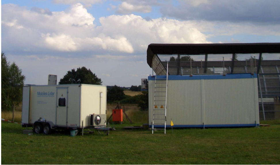
Figure 4.1: Measurement set-up of the ALADIN Airborne Demonstrator (container, right), the backscatter lidar MULIS (trailer, left), and the 482 MHz wind profiler (background right) at the Richard-Aßmann-Observatory, Lindenberg, in July 2007.
