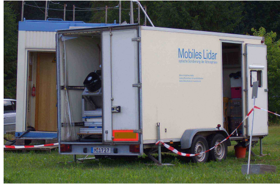
Figure 4.2: Aerosol backscatter lidar MULIS set up in trailer.
