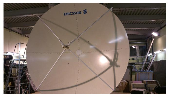
The antenna fulfil very demanding requirements concerning low side lobes, high antenna gain, similar antenna gain in H and V and very good cross polarization isolation
