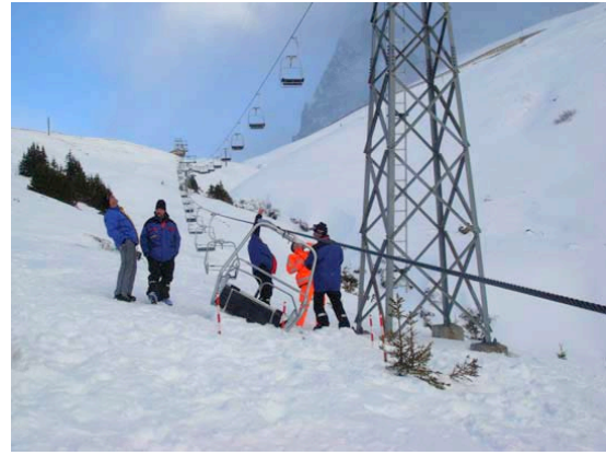
Figure 2. Chairlift accident. The cable was caught in the cable catcher, a subsequent gust threw it out. (Source: public UUS report)
