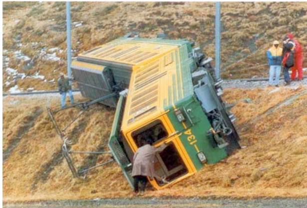
Figure 1. The motor coach after being derailed by foehn winds. (© Minirex AG, Schweizerische Eisenbahn-Revue)
