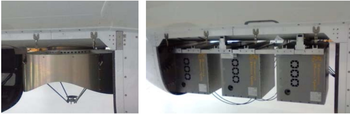
Figure 4.2 Left image: Cloud radar 35 GHz. Right image: Microwave radiometer 90/119, 22/58, 183 GHz mounted in Belly-Pod beneath the aircraft.
