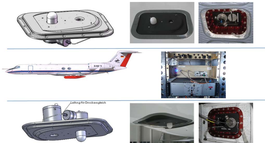
Figure 4.7 Images and illustrations of HALO-SR as mounted on HALO.
