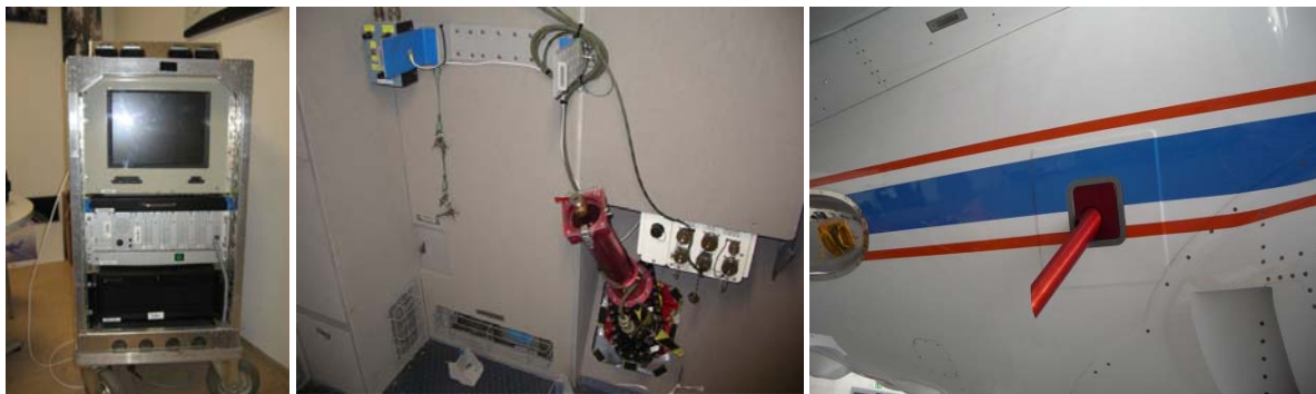
Figure 4.10 Left: Dropsonde data acquisition rack. Middle: release unit in HALO baggage compartment. Right: release pipe as seen from outside the aircraft.
