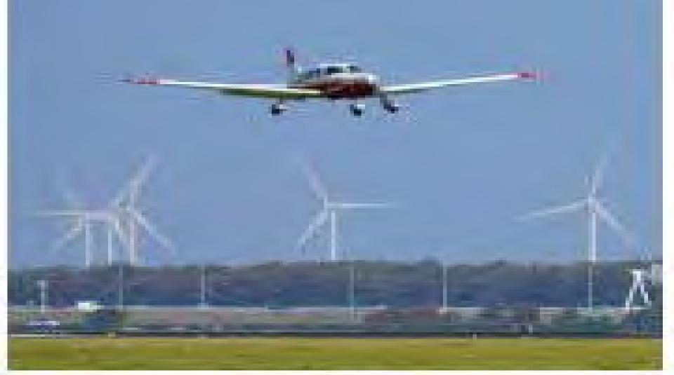
The risks of the wind turbines near the airport are not just wake effect problem but also the effects on radar. Wind turbines cause radar clutter that is very important for air traffic or create ghost images.
