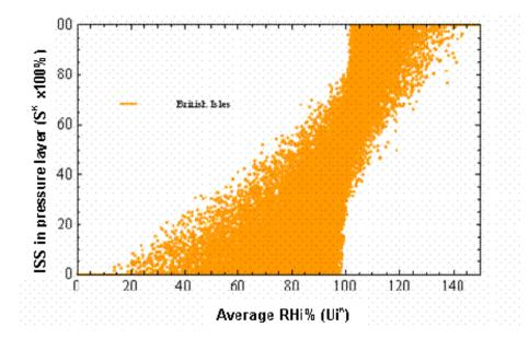
Figure 3. The fraction of humidity measurements indicating ice supersaturation vs. the corresponding average relative humidity wrt ice for 50 hPa pressure layers over the British Isles. These data have been grouped together in 5% RHi bins, and the mean of the fractional ISS occur-
