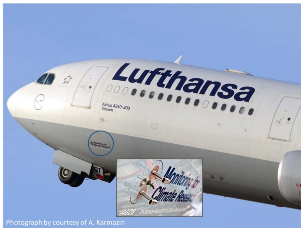
Figure 2. IAGOS-CORE installation position aboard the Lufthansa A340-300 “Viersen” (photograph by courtesy of A. Karmazin); the insert shows details of the IAGOS Inlet Plate which carries the inlet probes for trace gas sampling (photograph by courtesy of Lufthansa).
