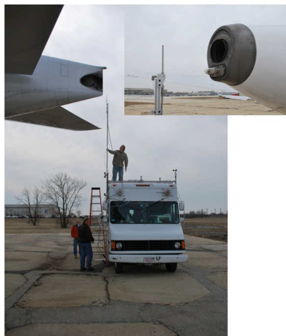
Figure 1. Aerodyne mobile lab preparing to sample the APU of a Boeing 777 as well as the sample inlet behind the exhaust port of an Airbus A320.
