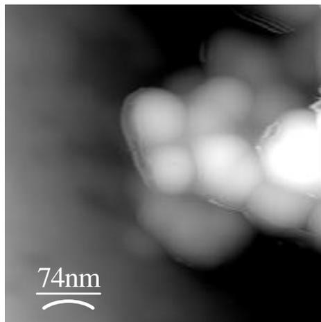
Figure 1. AFM image of engine soot
