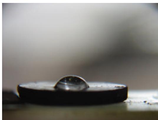
Figure 4. Water droplet on kerosene soot
