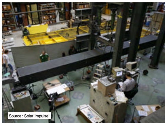
Fig. 5-15 Wing box, structural test
